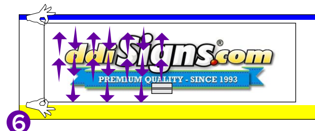
4 CUT THE BACKER AWAY. PERSON 1 HOLDING THE DECAL CAREFULLY MOVE TO THE RIGHT HOLDING THE DECAL AWAY FROM THE DASHER BOARD.
