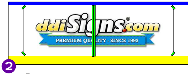
1 ALIGN THE DECAL ON THE BOARD WHERE YOU WANT TO INSTALL. TAPE THE CORNERS TO HOLD IN PLACE.
